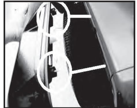
Step 8. Installing the rear flares. Install the rear fender flares using a 7mm rubber spacer on each screw. Mount the flare on the body placing a M5 nut on each bolt. Finally tighten the nuts. Do not over tighten the mounting nuts.
